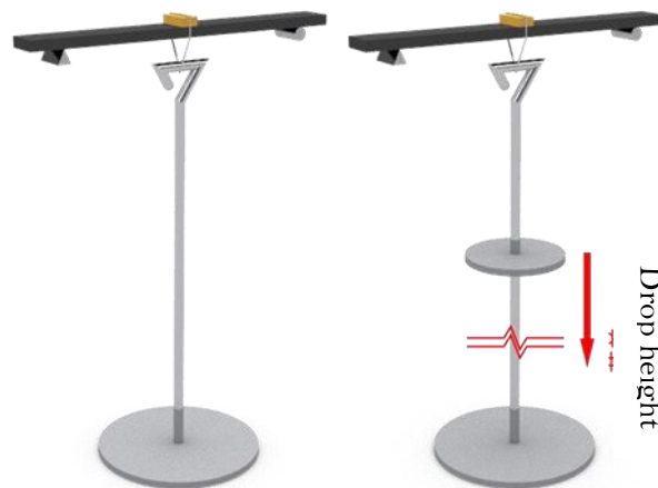
Figure-3. Loading test device schematic (Left: static load (recommended); Right: Impact)
