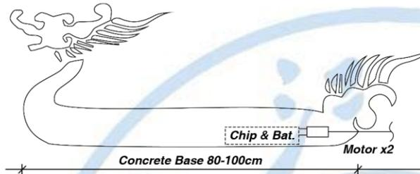
Figure-1 Model dragon boat hull size
