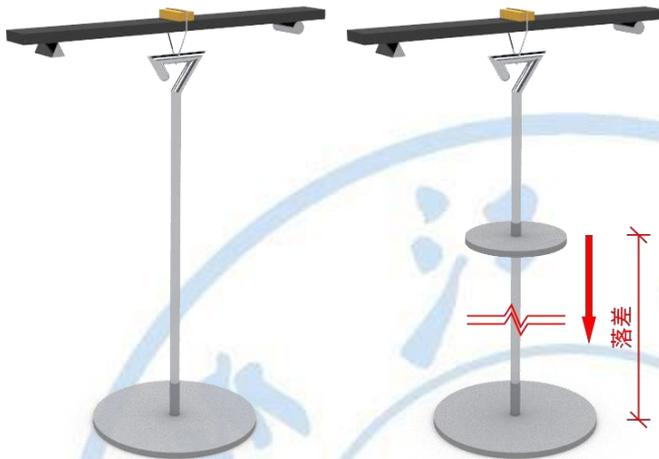
Figure-4 Schematic diagram of loading test device (left: static load; right: impact)
